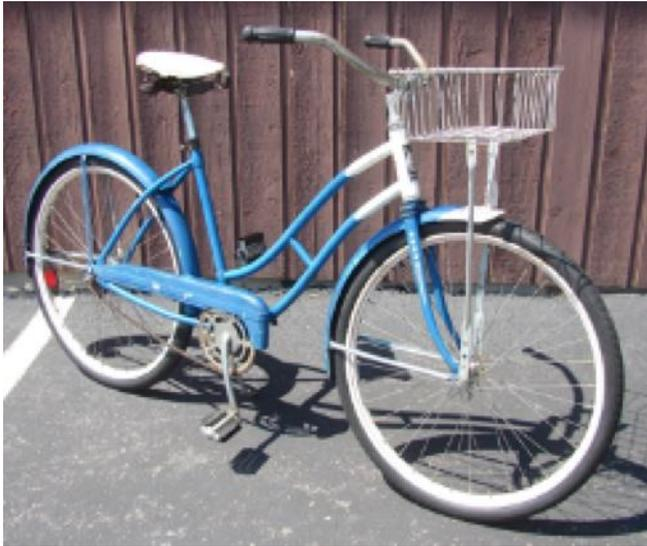
Manufacturing in Westfield Massachusetts. The bikes featured American made steel, coaster brakes and a single speed drive.
