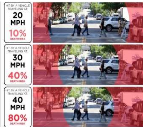
Figure 1. The effect of speed on a driver's field of vision and the risk of pedestrian death (Photo credit: LADOT)
